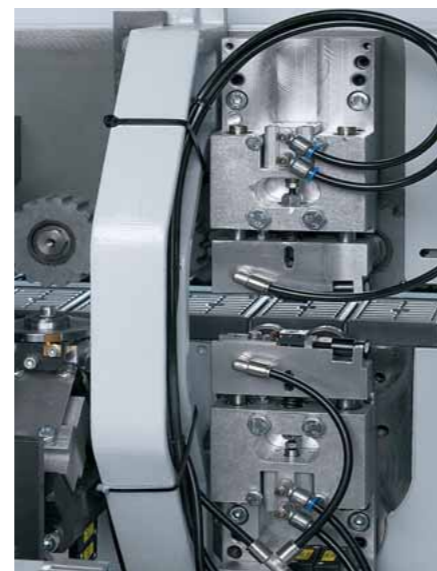
Glue joint scraping unit (optional) For the perfect finish.
